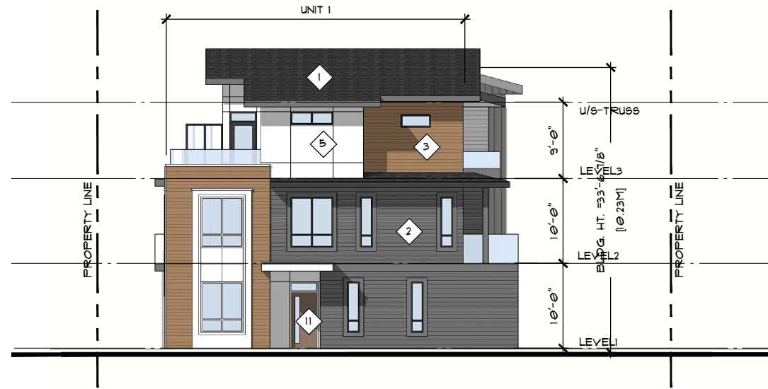
SOUTH ELEVATION - RAYMER AVENUE SCALE: 1/16"=1'-0"
